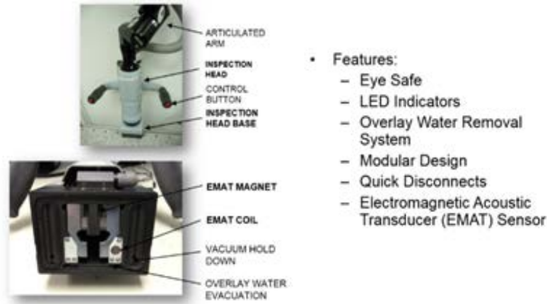
Figure 2: LBI inspection head.
