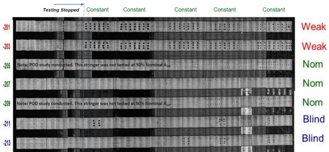
CFRP 1 Configured Demo 3.5 MHz, 64 Element Linear Array, Olympus OmniScan MX2 and glider with VACRS scan system
